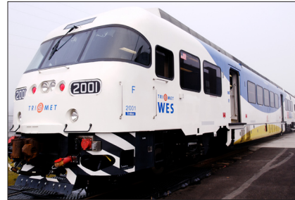
WES service debuted with four diesel multiple unit (DMU) vehicles.
