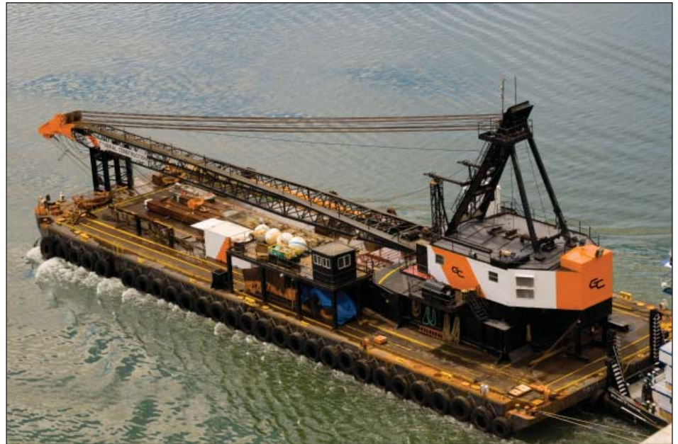
Figure 1.3 - A derrick barge is a crane mounted on a barge (DB-LA) will be used for the PMLR Bridge construction.
